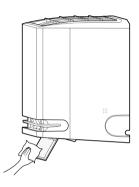
f 4 Press and hold the  $\c 3m$  button for about 5 seconds to close the air deflector.
