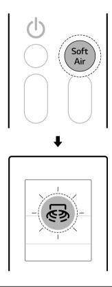
When connected to the Multi Outdoor unit, you cannot adjust the airflow temperature.
