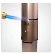
• Apply heat, keeping the flame moving to ensure that parent metals are evenly heated to a cherry-red colour.
